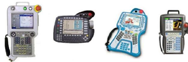
**Figure 4. Four teach pendants used for robot programming.**
